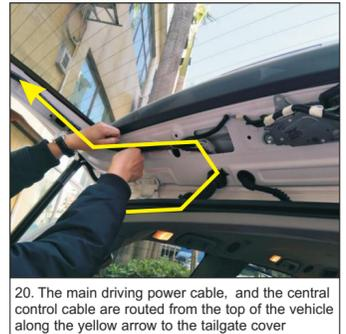
20. The main driving power cable, and the central control cable are routed from the top of the vehicle along the yellow arrow to the tailgate cover
