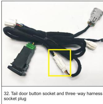
32. Tail door button socket and three-way harness socket plug
