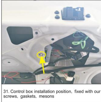
31. Control box installation position, fixed with our screws, gaskets, mesons
