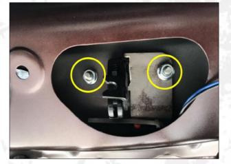
9.Remove the original car screw and fix the tailgate switch button bracket with the original car screw.
