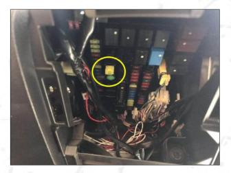
7.Remove the trim panel under the main driving, unplug the original car fuse, and plug in our power plug.
