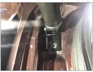
2.Remove the original left lower bracket, install our lower left bracket and fix it with our screws.
