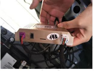
11.According to the color of socket, insert the plug into the control box.
