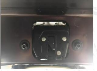
8.Remove the original car lock, install our electric lock.
