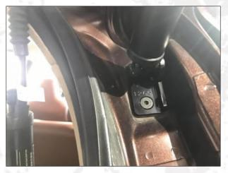
4.Remove the original right lower bracket, install our lower right bracket and fix it with our screws.
