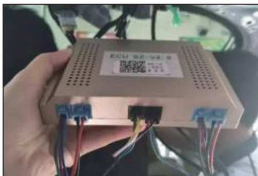
19. Hall wire, central control line and power cable are inserted into our control box one by one according to color.
