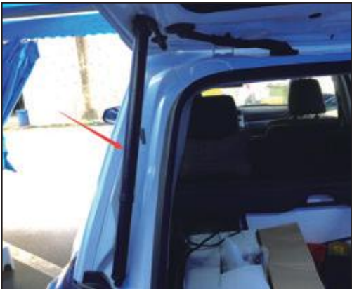
7. Installation of left and right electric pole is completed
