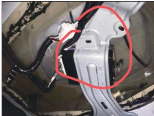
17. The control box is attached to the black color box of the original car. Secure with a tie.
