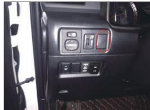
15. Remove the original car switch and install the tailgate switch under the main driver compartment
