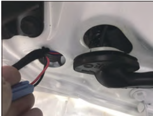
8. Install electric pole wiring on the original vehicle
