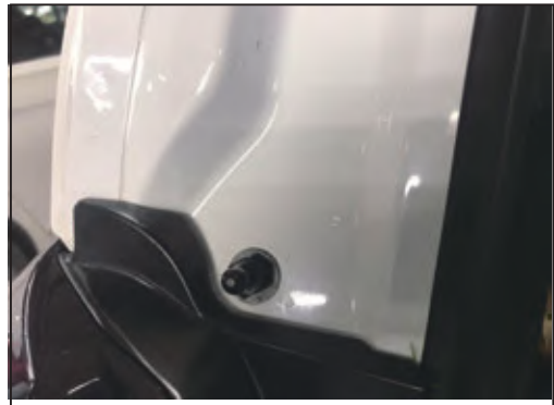
3. Remove the lower ball head from left and right of the original car.
