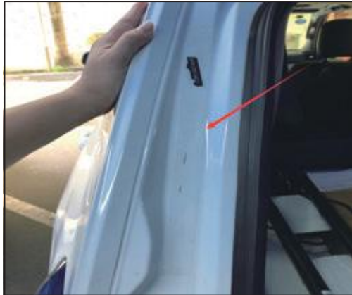
5. Paste our anti-collision sticker on the original car (left and right alike)
