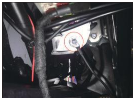
12. Connect grounding under the steering wheel of the original car
