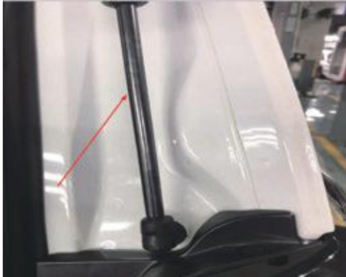
2. Remove the right support pole of the original car
