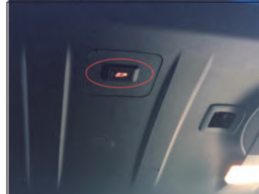
15. Remove the original car switch and install the tailgate switch under the main driver compartment
