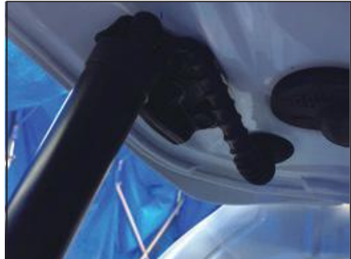
3. Remove the lower ball head from left and right of the original car.
