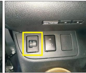
11. Remove the original car small lamp terminal housing
