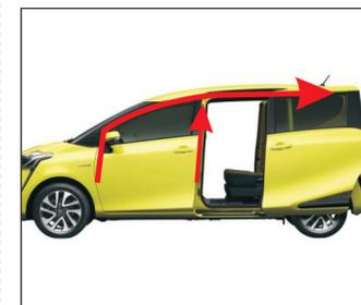
17. The main driving power cable, front switch cable and central control wire pass through the waterproof rubber plug along the yellow arrow to the tailgate cover.
