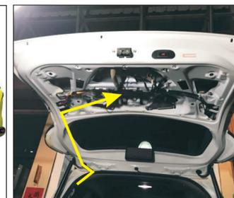
18. The power cable, front switch wire and central control wire pass through the waterproof rubber plug along the yellow arrow to the tailgate cover.
