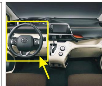
9. Remove the trim panel under the main driver and find the original car power supply.
