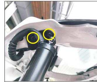
2. Remove the left upper bracket of the original car and install the left upper bracket of our company. The ball head is facing the tailgate and fixed with our screws
