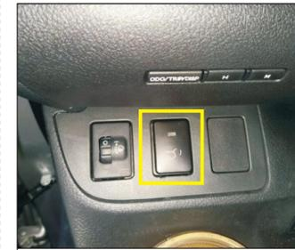
10. Remove the original car empty button at the main driving steering wheel as shown in the figure, and install the front switch button of our company.
