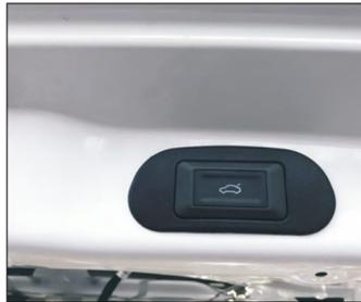
32. Remove the plaque and punch the hole and install the tail button of our company. The tail door socket and the socket of the three-way harness are inserted.
