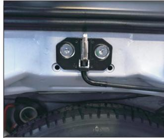
24. Remove the original car lock, install our electric shock lock, and fix it with our screws.
