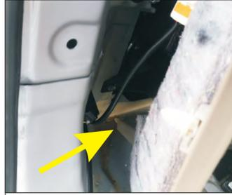
26. The motor is installed on the left side of the tailgate and fixed with our 3M glue.
