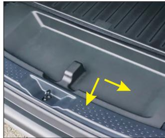
22. Take out the load plate at the tailgate, remove the plaque, and find the original car lock.
