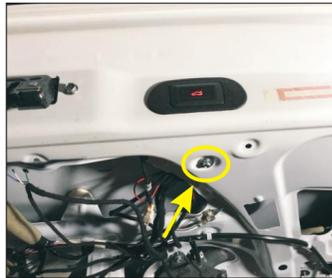
31. Control box installation position, fixed with our screws, gaskets and mesons
