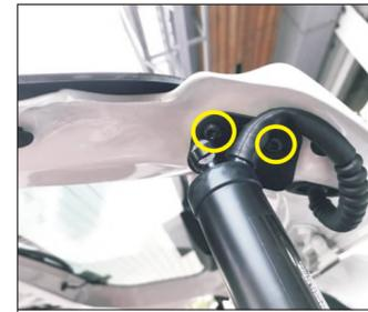
4. Install the upper right bracket of our company, and the ball head is facing the tail door. Use our screws to fix the right upper bracket of the original car.
