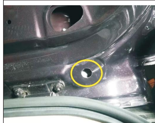
3. Remove the tail door trim, right brace body dozen 16 mm hole, hole thread through the hole line
