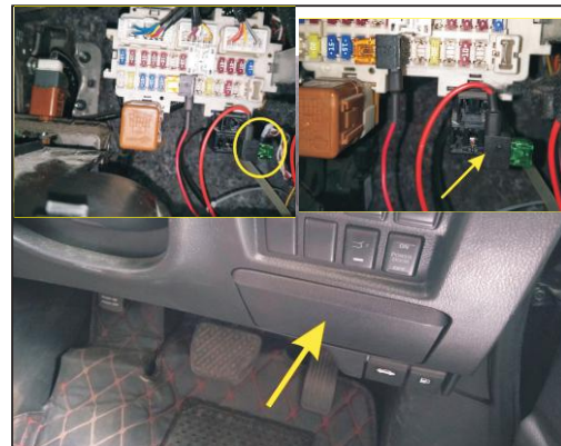
7. Remove the plaque, the main driving below the original car a hole location on the right with our power plug
