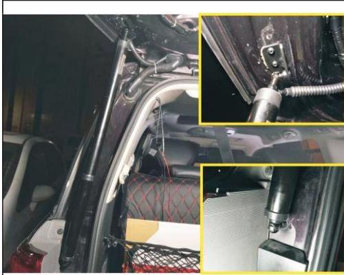
1. Remove the original car left brace and bracket, installation dedicated stent, ball head and brace, use our screws
