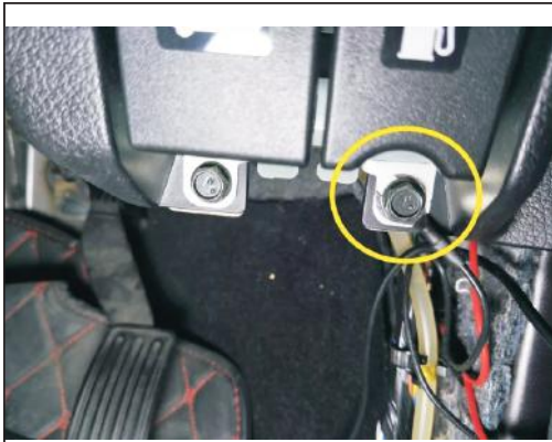
8. Below the power supply, our earth grounding screw
