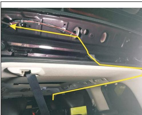
12. And the power cord, switch before the Central Line away from the main driving line to end door cover plate
