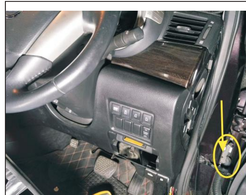
10. Main driving car door in the original car door stopper is pulled up
