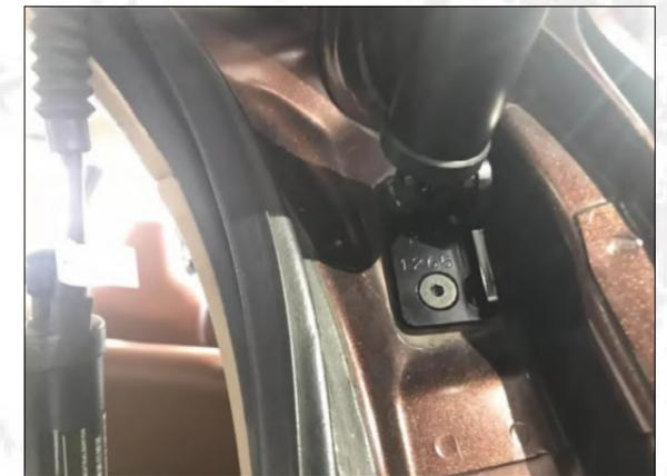
4. Remove the original right lower bracket, install our lower right bracket and fix it with our screws.
