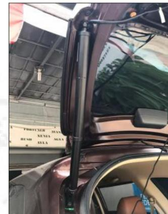
5. Installation completion diagram.
