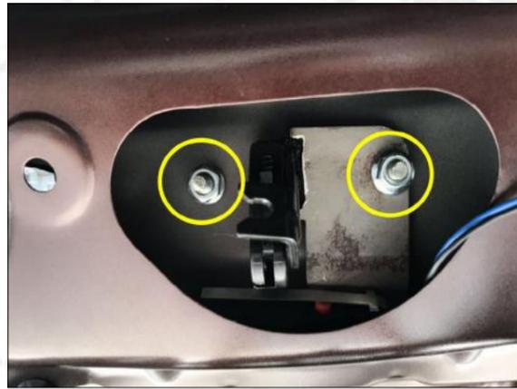
9.Remove the original car screw and fix the tailgate switch button bracket with the original car screw.
