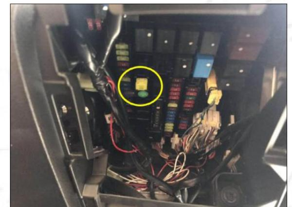
7. Remove the trim panel under the main driving, unplug the original car fuse, and plug in our power plug.
