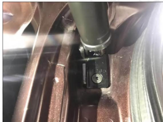
2. Remove the original left lower bracket, install our lower left bracket and fix it with our screws.
